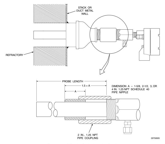
Figure 2-5. Adjusting Probe Insertion Depth
